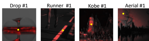
Fig. 5. Selected attention maps of the first frame. Yellow points denote the pixels randomly selected from each image, and red areas denote the active places.
